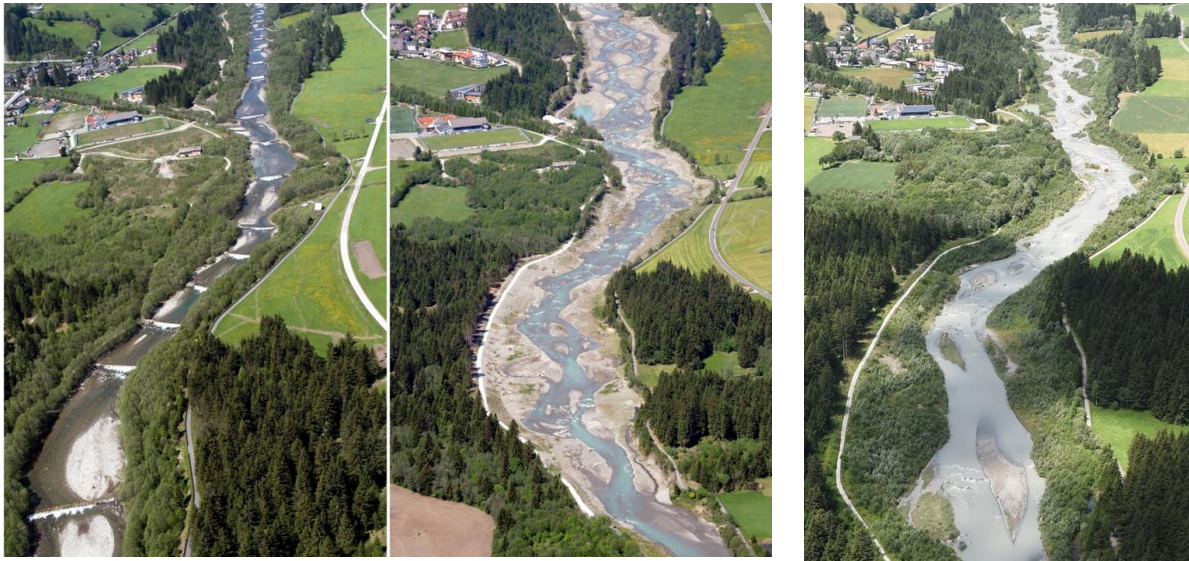
Fig. 16: Rio Mareta before (left) and immediately after restoration (mid); and ten year after restoration (right). Note in the right picture the alluvial forest established on brand new flood plain recreated by the river.
