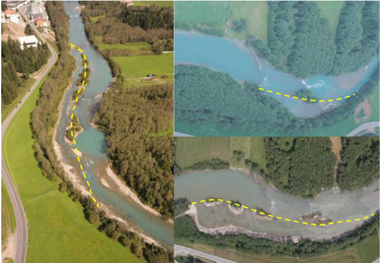
Fig. 17: Examples of interventions. Dashed yellow lines indicate the position of former bank, before river-bed enlargement.
