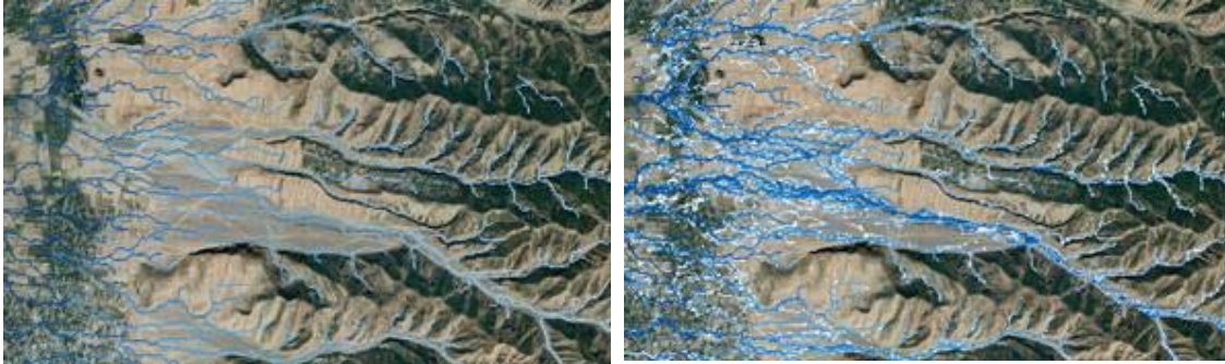
Figure 7: GIS-based flash flood and mudflow trajectory analysis (Lohr, 2018)
