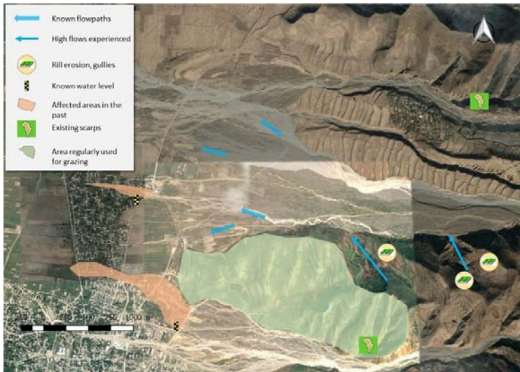
Figure 8: Example of a simple flood inventory map based on knowledge from past events
